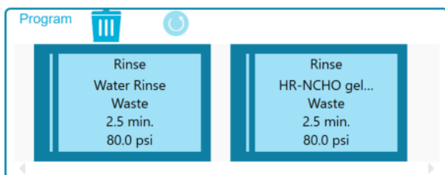
Figure C-6 Actions in the Program Pane for the Conditioning Method
