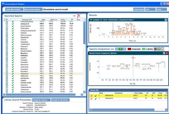
Figure 6. Automated library confirmation for Salbutamol from a hydrolyzed urine sample after DPX cleanup.
