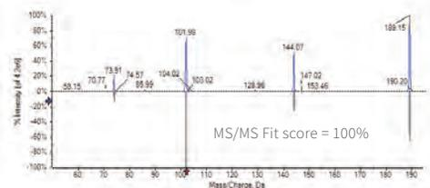
QTRAP technology enables collection of high-quality MS/MS spectra in addition to MRMs to enable library comparisons for better confidence in compound identification.
