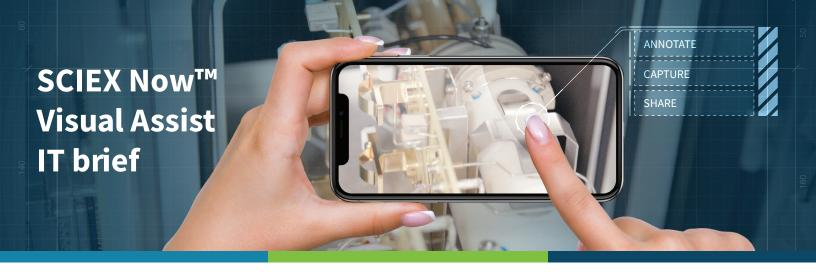
SCIEX Now™ Visual Assist is an augmented reality (AR) powered technology integrated into the SCIEX Now™ service call management system. This technology allows SCIEX Now Technical Assistance Center (TAC) specialists to visualize the issue on the customer's system through a mobile phone and perform activities such as annotate, zoom in/out of still images and capture video.
