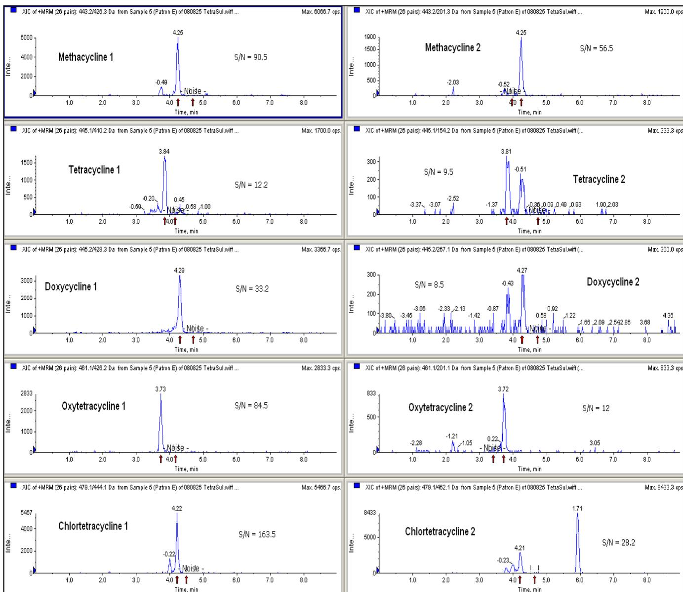
Figure 2. Example chromatograms for a spiked matrix standard at 0.5 ppb equivalent to 50 ppb in meat (signal-to-noise measured using PEAK:PEAK script on unsmoothed raw data).
