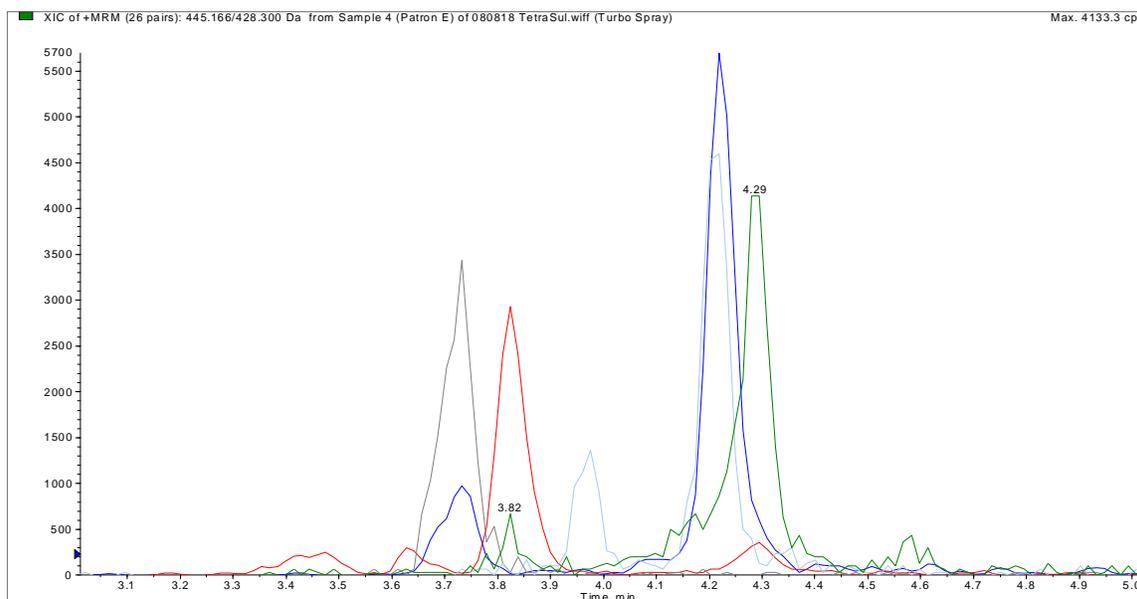
Figure 1. Example chromatogram for a spiked matrix standard at 0.5 ppb equivalent to 50 ppb in meat, showing all the tetracyclines overlaid in one window (between 3 and 5 minutes). The analytical run is 9.0 minutes.
