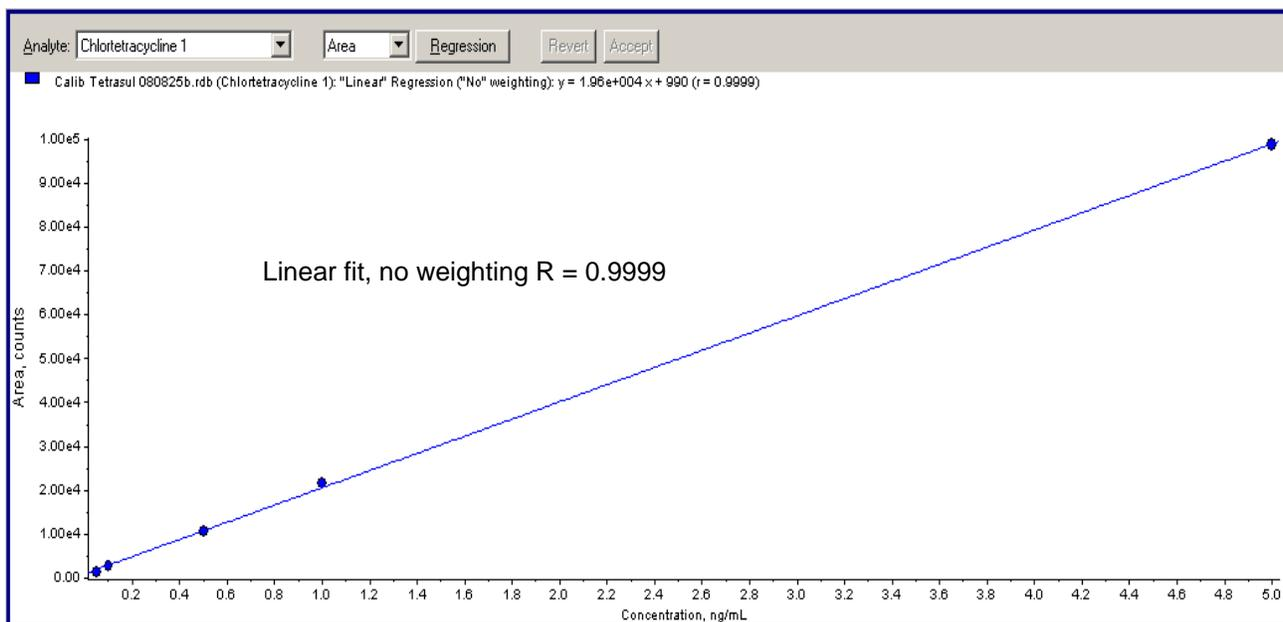
Figure 4. Calibration line for chlortetracycline 1, standards 0.05 to 5 ppb (no internal standard used).
