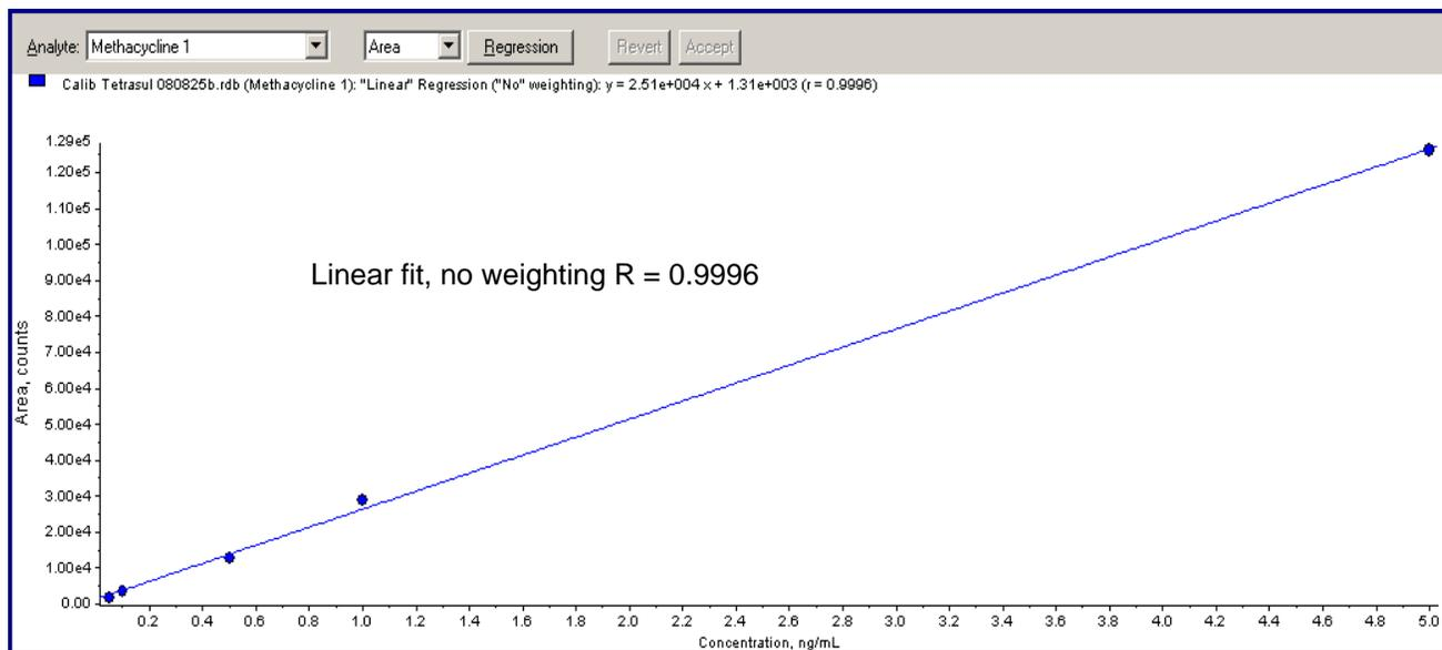
Figure 3. Calibration curve for methacycline 1, standards 0.05 to 5 ppb (no internal standard used).
