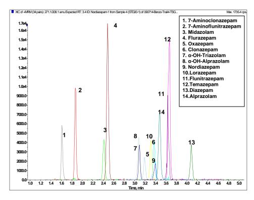
Figure 1. Representative chromatogram of spiked urine at 20 ng/mL performed on a 3200 QTRAP® LC/MS/MS system with a Shimadzu LC system in a 8.3-minute run
