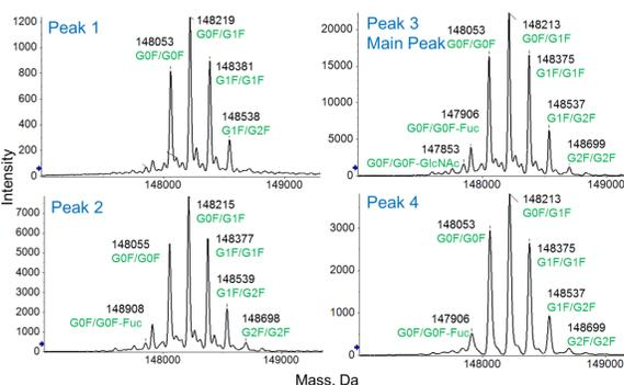
Figure 3. The deconvoluted spectra of each of the four CESI-MS peaks
