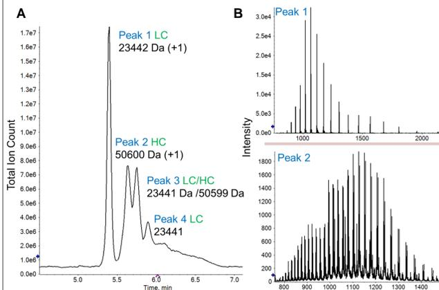
Figure 4. A. The separation profile of Trastuzumab subunits. B. The protein envelopes of Peak 1 and Peak 2 respectively.
