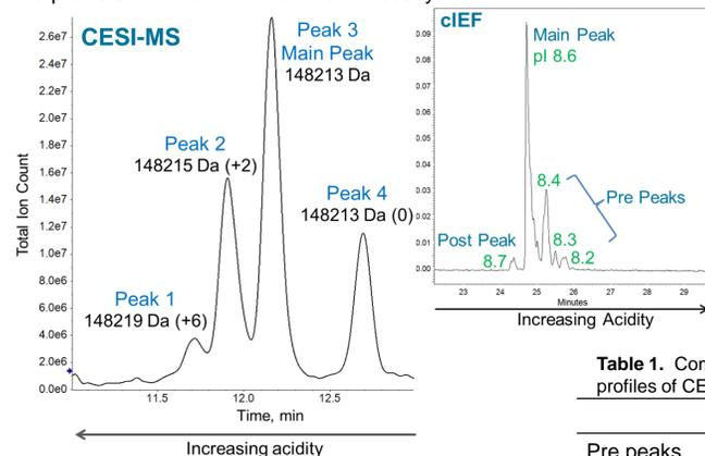
Figure 2. CESI-MS peak profile of Trastuzumab. Insert is the cIEF of Trastuzumab.
