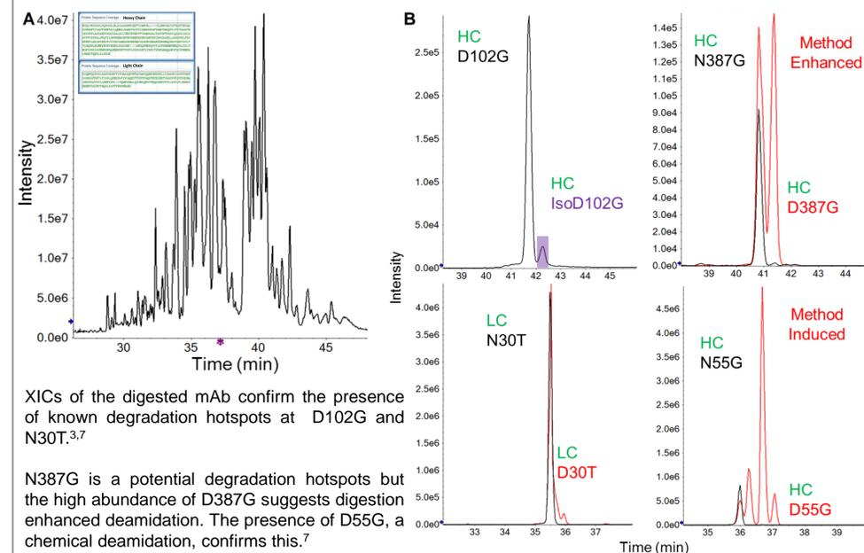
XICs of the digested mAb confirm the presence of known degradation hotspots at D102G and N30T.<sup>3,7</sup>
