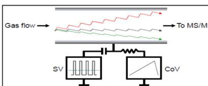
**Figure 1. Differential Mobility Separation Process.** Innovative planar design of the DMS cell uses an asymmetric RF waveform (SV) to separate ions based on differential mobility between the high and low fields. The compensation voltage (CoV) is used to correct the trajectory of the ion of interest which traverses the cell and into the orifice while interferences are deflected into the cell walls.
