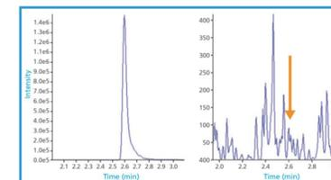
Figure 6. Carryover for insulin glargine after injecting the extract of a sample spiked at the 10,000 pg/mL level. Carryover based on peak intensity was less than 0.01%, and low enough to declare 10,000 pg/mL as the ULOQ.
