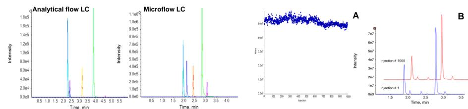
Figure 3. XIC Chromatograms for the analytical flow LC-MS method (left) and the Trap-and-Elute Microflow LC-MS method (right) for the infliximab and IS signature peptides.
