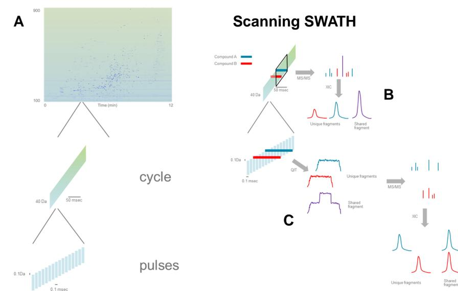
Scanning SWATH acquisition. During each cycle, the isolation window for MS/MS is sliding along the m/z range of interest. At each pulse, the isolation window is shifted slightly higher in m/z. The data from every pulse is stored (section A).
