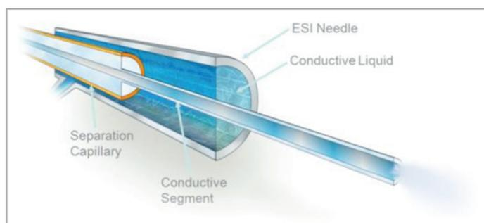
**Figure 1.** The OptiMS cartridge provides an ultra-low-flow ESI interface.
