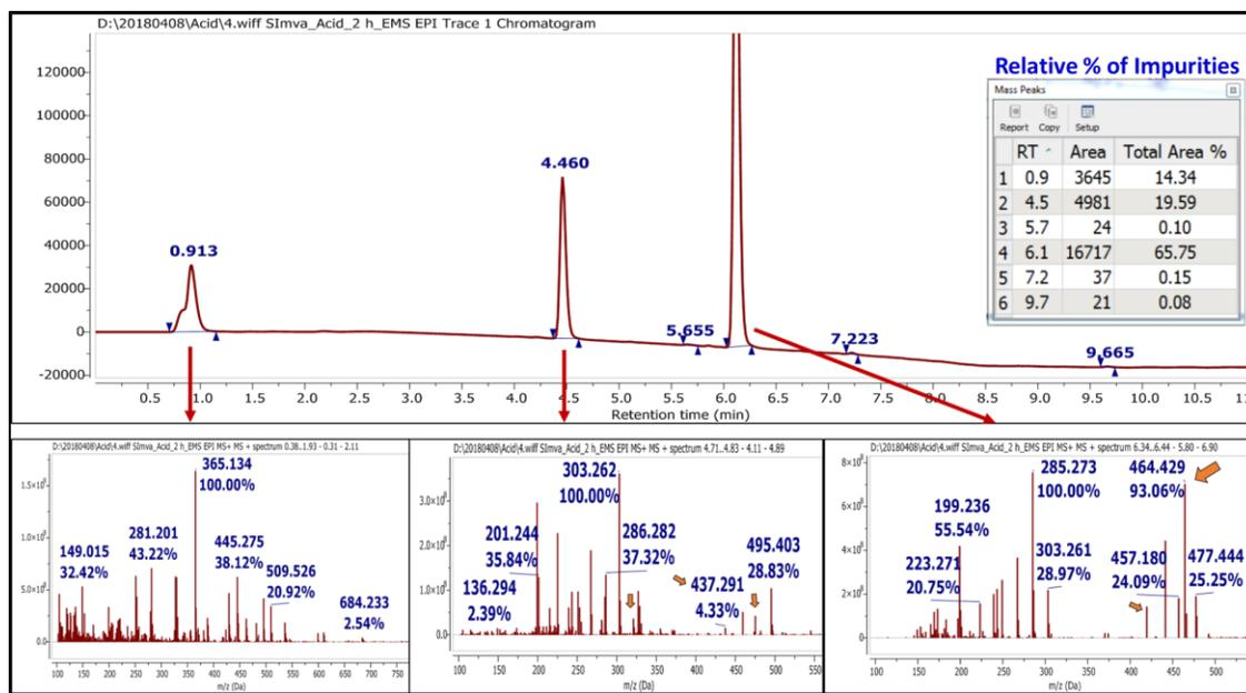
**Figure 5. UV Data Processing by Using Mnova MS Software.** UV signals from the major components are shown (top) and the relative % based on UV area is computed (inset). (bottom) The MS spectra extracted at the retention times of the major UV peaks (0.91, 4.46 and 6.9 mins) are shown.
