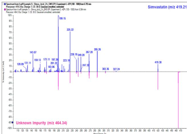
**Figure 4. Comparison of MS/MS Simvastatin (m/z 419.21) to Coeluting Impurity (464.34).** MS/MS matching shows majority of fragment ions are the same, suggesting a structurally related degradation product.
