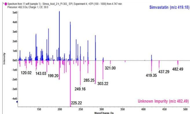
**Figure 8. Comparison of MS/MS Simvastatin to Impurity Detected from Precursor Ion Scan Experiment.** MS/MS matching shows many similar fragment ions are the same, again suggesting a structurally related degradation product.
