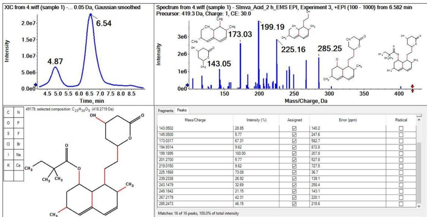
**Figure 6. Identification of Common MS/MS Fragments from Simvastatin.** The high-quality MS/MS spectrum of simvastatin generated using the EMS to EPI workflow was compared with the theoretical product ion spectra generated using simvastatin's mol file in the PeakView software and compared for similarity check.
