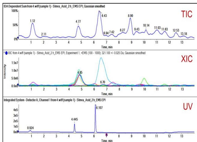
**Figure 3. Profiles of Simvastatin Sample.** Total Ion chromatogram (TIC), extracted ion chromatogram (XIC) of major degradation products and UV profile of Simvastatin (Acid hydrolyzed) sample.
