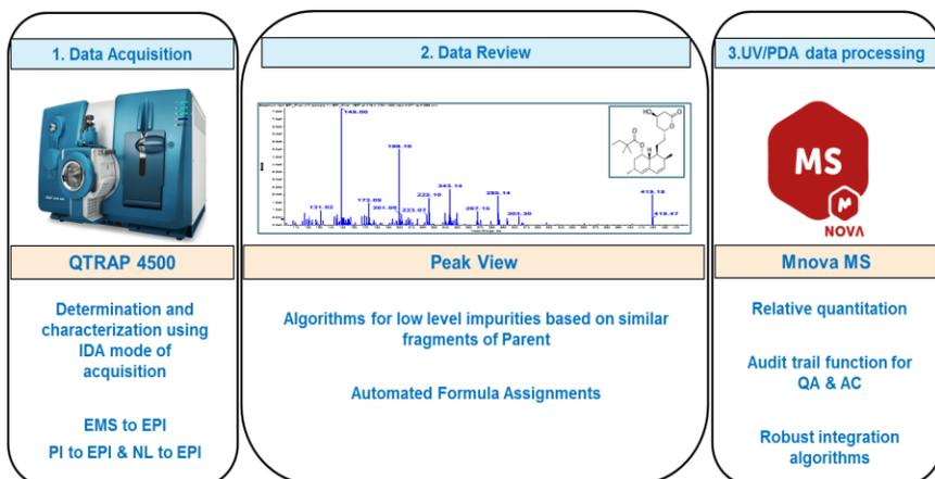
**Figure 1. Impurity Profiling Workflow.** Data Acquisition using QTRAP® 4500 system, both untargeted survey scans (EMS) and targeted survey scans (Precursor ion PI and Neutral loss NL scans) were used to trigger EPI (full scan MS/MS) data for identification. Data processing was performed using PeakView® Software to identify the components. Finally, UV/PDA data was processed using Mnova.
