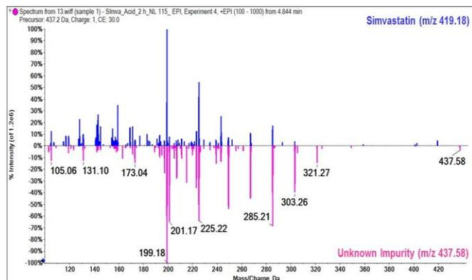
**Figure 10. Comparison of MS/MS Simvastatin to Impurity Detected from Neutral Loss Scan Experiment.** MS/MS matching shows many similar fragment ions are the same, confirming detection of Simvastatin Acid.
