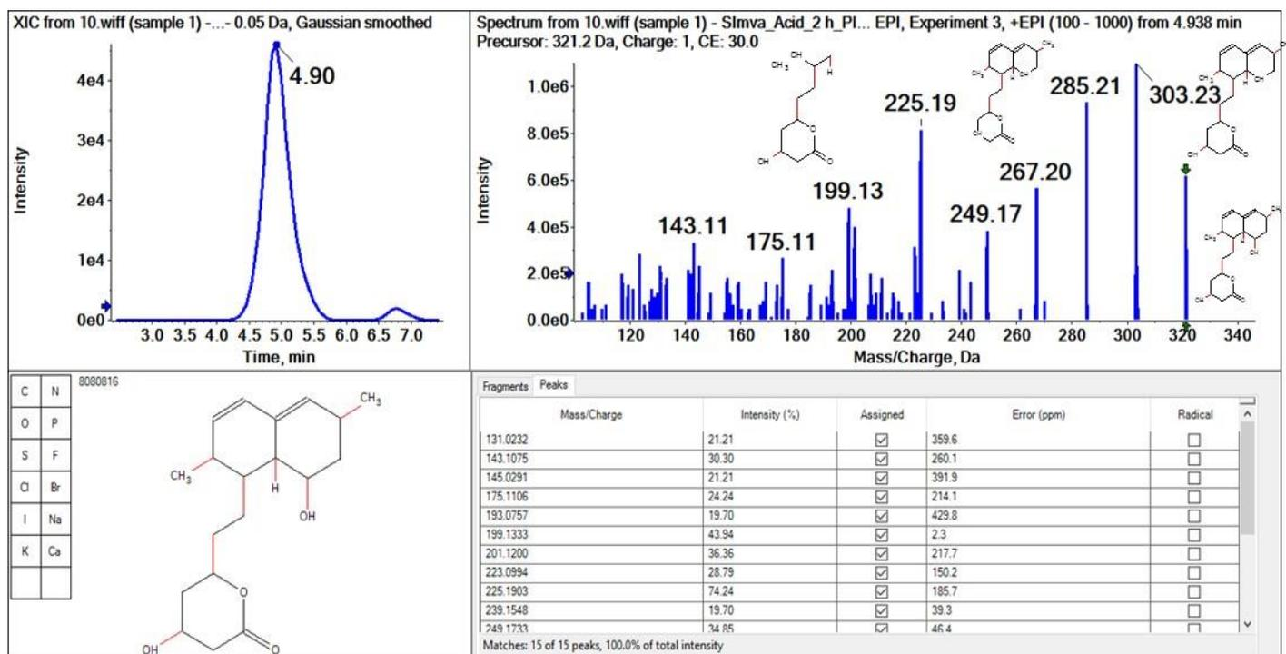
**Figure 7. MS/MS Confirmation of Structurally Related Known Impurity (Simvastatin Lactone Diol).** The high-quality MS/MS spectrum of simvastatin lactone diol generated using the EMS to EPI workflow was used compared with the theoretical product ion spectra generated using mol file in PeakView software and compared for similarity check.
