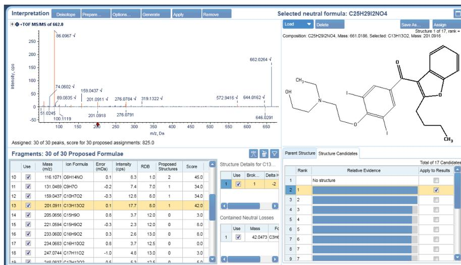
**Figure 11. MetabolitePilot Software Interpretation of Amiodarone Oxidation Impurity Isomers.** The interpretation workspace of MetabolitePilot software displaying results of the 14.2 min amiodarone-oxidation peak, and the top structural proposal. The MS/MS fragment at 201.09 shows there is no oxidation on the butyl-benzofuran moiety and establishes that oxidation is occurring on the other side of the molecule
