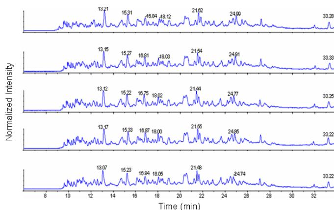
**Figure 4. Reproducibility of Ionization.** Replicate injections of a 20-protein mixture were performed and the MS TIC was compared across the samples. A commercial C18 nanoLC column (150 x 0.075 mm, 350 nL/min) was used with a 10  $\mu$ m ID emitter tip (length: 7cm). Good TIC reproducibility was observed.
