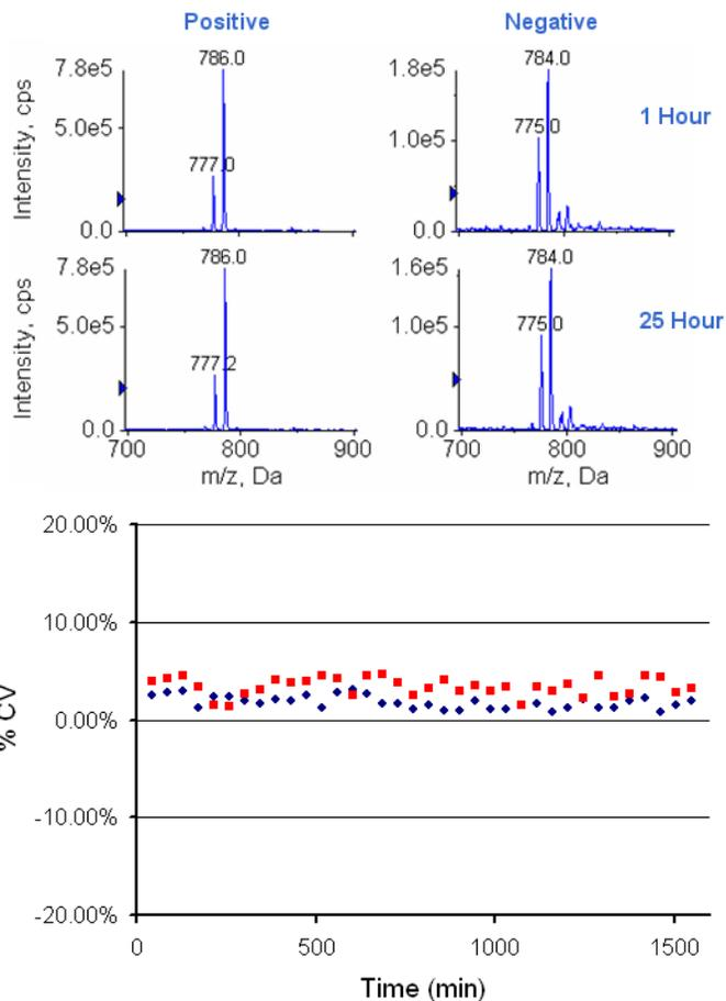
**Figure 7. Stability of Polarity Switching.** Shown in top panel are the Q1 spectra for Glu-Fibrinopeptide B in + and – mode during 3 sec polarity switching cycles. Below are the identical spectra after 25 hours of continuous polarity switching experiments. The %CV from the positive (blue circles) and negative (red squares) signals from 0-25h throughout the experiment are plotted in the bottom panel.
