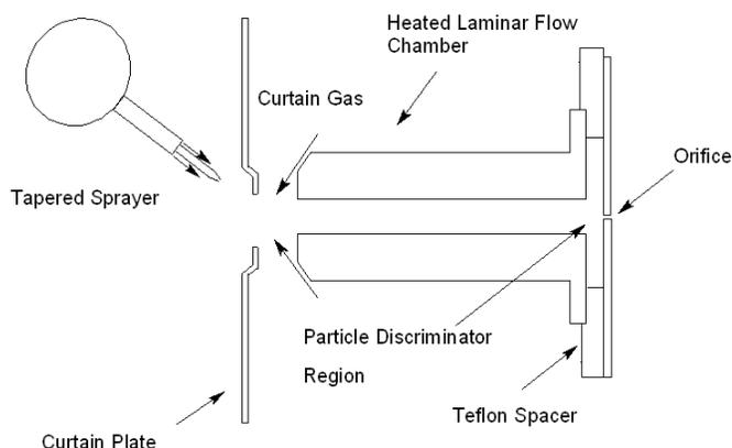
**Figure 3. Schematic of Heated Interface.** Ions are generated within a few millimeters of the entrance to the heated laminar flow chamber. Two stages of desolvation are provided with the Curtain Gas™ interface and heated chamber. More favorable gas dynamics are provided by reduction of the curtain gas flow speed and establishment of laminar flow prior to the gas conductance limiting orifice.
