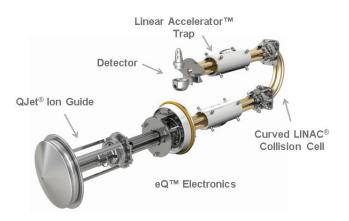
**Figure 1. QTRAP System Ion Rail.** The unique configuration of the QTRAP system consists of a triple quadruple-based ion rail, where the third quadrupole (Q3) can also operate as a linear ion trap (LIT). This configuration provides a broad range of traditional scan functions along with new and unique workflows that combine qualitative and quantitative data within one analysis without sacrificing performance.
