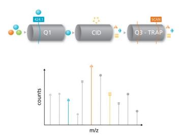
**Figure 6. Enhanced Product Ion Scan (EPI).** Precursor ions are selected in Q1, fragmented in Q2 using CAD, and then detected in the LIT. This unique QTRAP scan type will provide a high sensitivity full scan MS/MS spectrum of any precursor ion without the low mass cut-off typically observed with conventional ion trap instruments.
