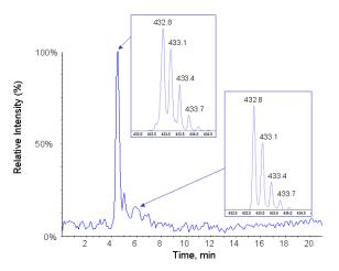
Figure 9. Dynamic Fill Time (DFT). Dynamic Fill Time carefully controls the number of ions that fill the linear ion trap so that optimum sensitivity and good resolution can be achieved across the LC-MS peak. Shown here is good resolution achieved at the LC peak apex where DFT automatically reduces the trap filling to reduce the chance of saturation (top) and good sensitivity obtained low in the peak tail where the trap is filled for longer (right).
