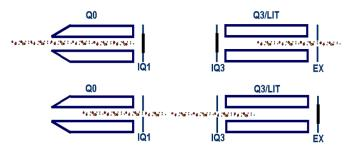
**Figure 8. Q0 Trapping.** Ions can be captured and stored in Q0 during trap scanning, reducing ion losses. When the trap is ready to be filled for the next scan, ions are released from Q0 and passed back to Q3. This can provide significant gains in sensitivity in EPI mode (MS/MS).
