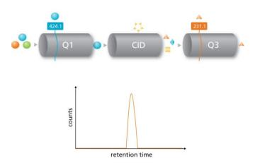
**Figure 2. Multiple Reaction Monitoring (MRM).** In this QqQ scan mode, a precursor ion is selected in Q1, it is then fragmented in the Q2 collision cell, and a specific product ion is monitored in Q3. The Q1 and Q3 quadrupoles are functioning in transmission only mode which means they are set to transmit a specific m/z only. This mode is what confers the high sensitivity of this scan as the instrument is fully optimized to transmit just that parent to fragment pair.
