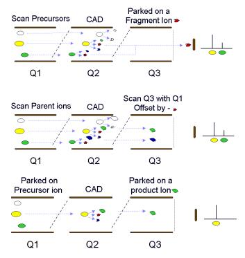
Figure 4. Triple Quadrupole Scan Types. Top – Precursor Ion scan. Middle – Neutral Loss scan. Bottom – MRM scan.
