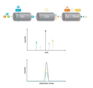
**Figure 3. MRM<sup>3</sup> Scan.** The precursor ion is first selected in Q1, then fragmented in Q2. Fragment ions are trapped and then isolated in Q3 which is now acting as a linear ion trap. This is followed by excitation to perform the second fragmentation step. Second generation product ions are then scanned out to the detector.
