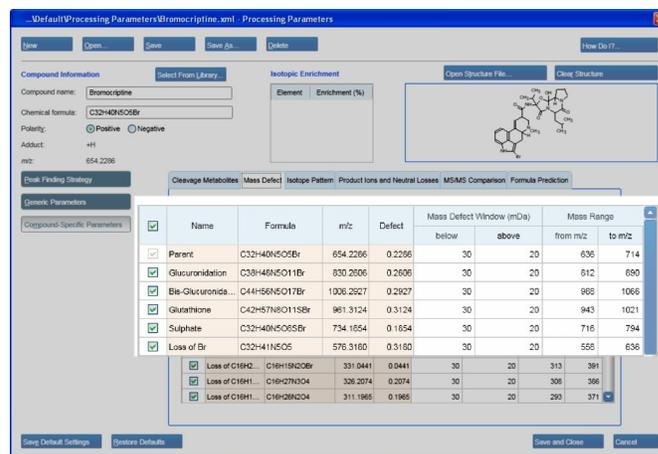
**Figure 1. Multiple mass defect filtering setup in the processing parameters.** MetabolitePilot™ software automatically calculates the mass defect filters for multiple metabolite classes using the parent structure.
