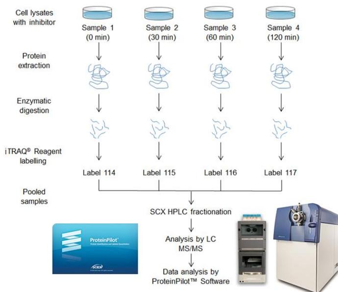
**Figure 2. Workflow for iTRAQ Reagent Labelling and Sample Analysis.** T47D breast cancer cells treated with IMD0354 were lysed, digested with trypsin, then labelled using iTRAQ reagents 4-plex. Labeled samples were mixed at equal ratios, and fractionated by strong cation exchange chromatography. 16 fractions were then analysed by LC-MS/MS using the TripleTOF® 5600 System. Proteins were identified and quantitated using ProteinPilot™ Software.
