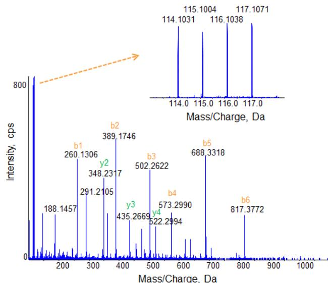
**Figure 3. High Resolution, High Mass Accuracy MS/MS Acquisition.** High quality MS/MS is acquired using high sensitivity mode using 200 msec accumulation time. Resolution of >15,000 resolution is typically obtained on the fragment ions and reporter ions ensuring confident identification and quantitation. The peptide shown is DELADEIANSSGK from Myosin-9 (546.28  $m/z$ ).
