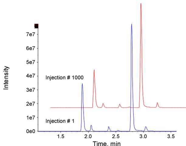
**Figure 5.** Total Ion Chromatograms for injection 1 and 1000 of the robustness test. Separation and peak shapes are identical.
