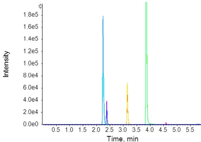
**Figure 2A, XIC chromatogram for the High Flow LC-MS method.**
