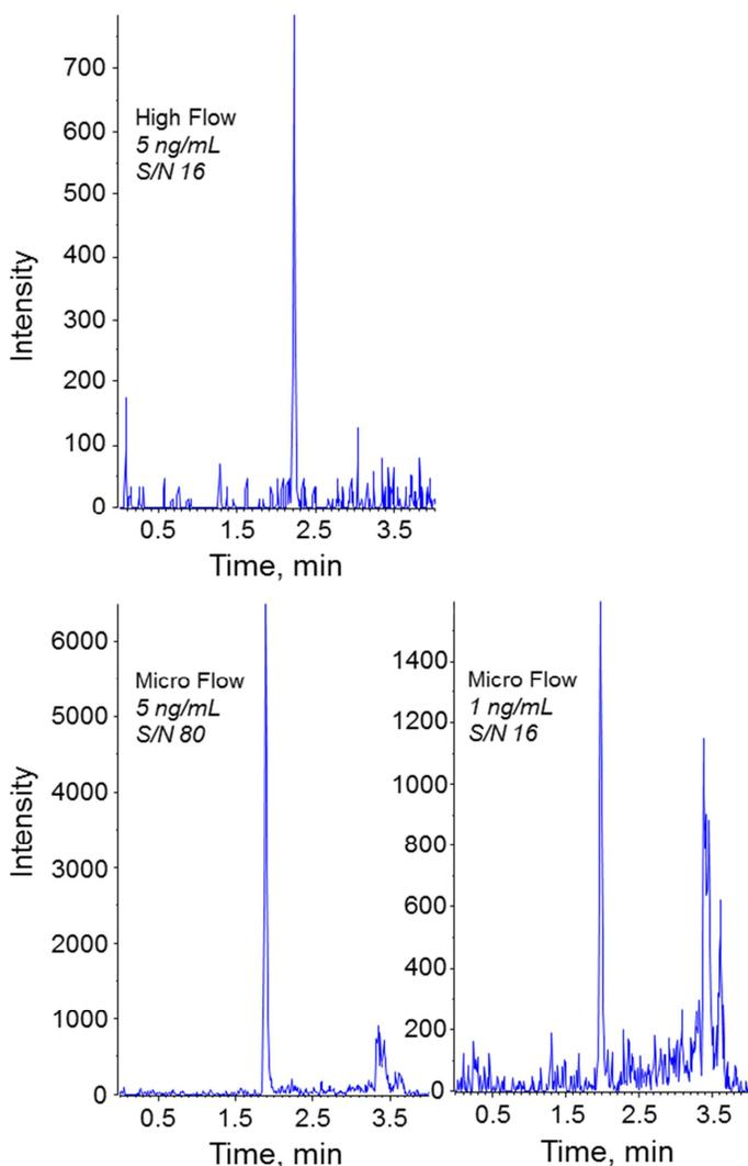
**Figure 3. Sensitivity comparison between the High Flow LC-MS and MicroLC trap-elute methods.**
