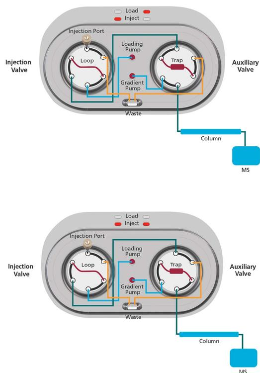
**Figure 1. Valve positions for the trap loading part of the method (top) and the analysis part of the method (bottom).**
